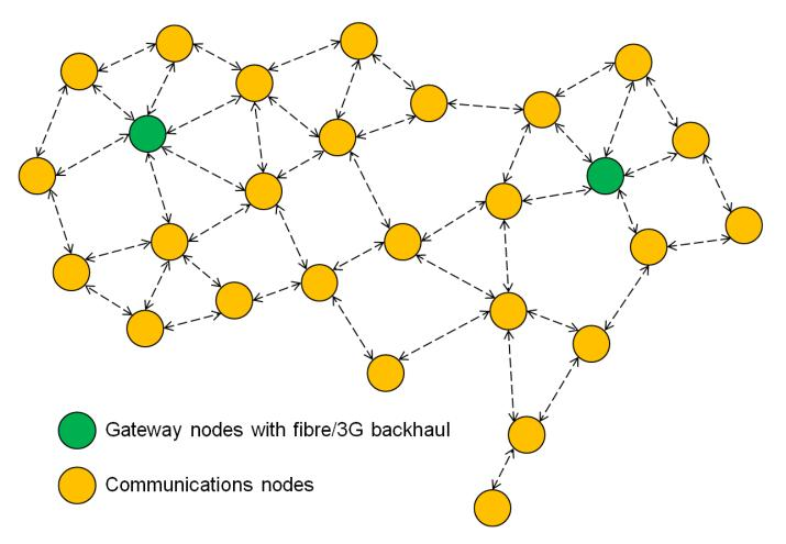
A TV White Spaces (TVWS) communication system with mesh networking capabilities has been developed to support autonomous collation of data captured by sensors attached to power grid infrastructure such as OG boxes or distribution substations and low voltage substations.
